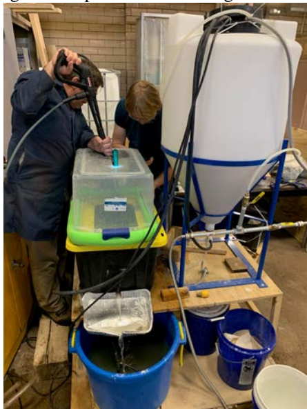
Figure 1: Gypsum-saturated excavation test setup
